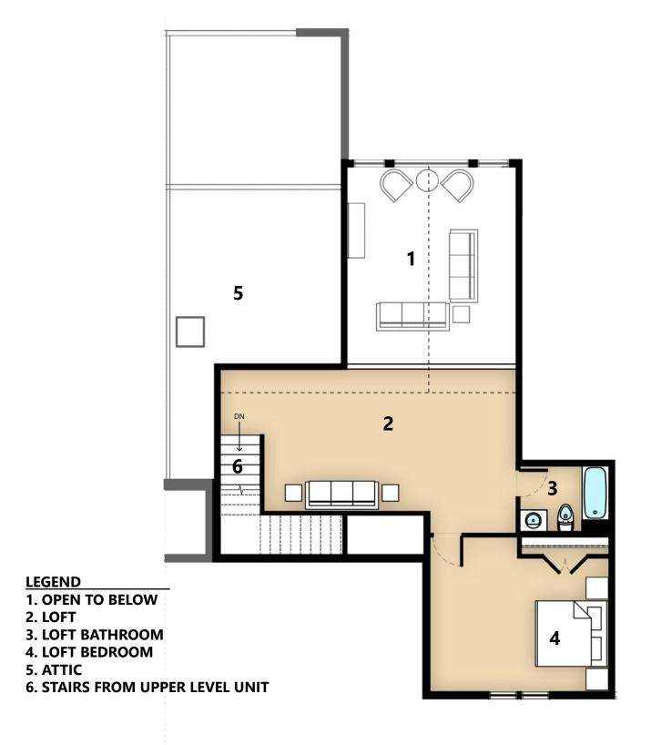
**UPPER LEVEL LOFT UNIT FLOOR PLAN** SCALE 1/8"=1'-0" SF: ~635
